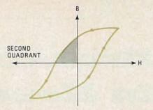
FIG. 2—THE DEMAGNETIZATION CURVE corresponds to the second quandrant of the hysteresis curve.
