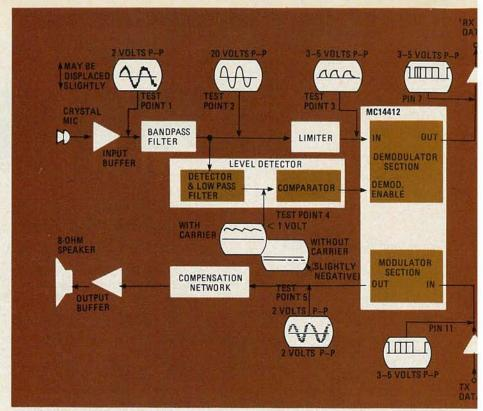
FIG. 1—BLOCK DIAGRAM OF the modern. The scope patterns shown are those that should be observed at the test points shown on the schematic (Figs. 1 and 2).
