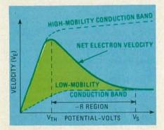
FIG. 2—AT POTENTIALS GREATER than V<sub>TH</sub>, an increasing number of electrons are scattered into the low-mobility conduction band.
