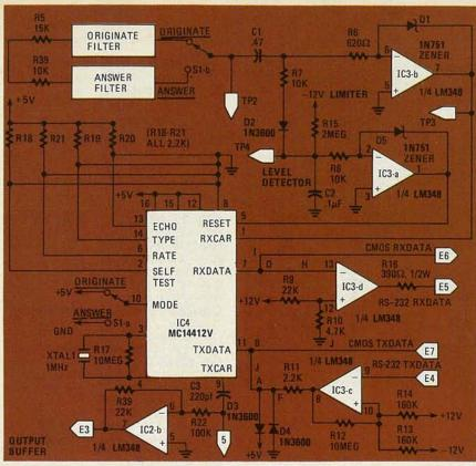
FIG. 3—HEART OF THE CIRCUIT is the MC14412 that performs all the modulation/demodulation
