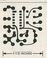
FIG. 93—YOU CAN ETCH detector board yourself from this pattern. Ready-made boards are also available (see parts list).
