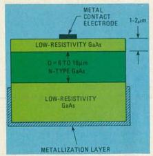
FIG. 3—THE GUNN DEVICE shows a diode-like structure although it is not a PN junction.
