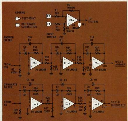
FIG. 2—THREE-STAGE ACTIVE FILTER (IC1-b, -c, -d and IC2-a, -c, -d) attentuates out-of-channel noise.
