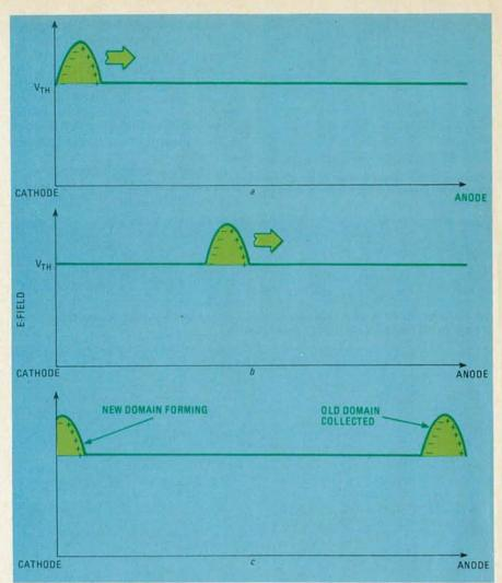
FIG. 4—WHEN the Gunn device is biased at V<sub>TH</sub>, a domain builds up at the cathode end (a), drifts through the Gunn device (b), and is collected at the anode (c).
