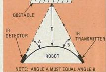
FIG. 88-INFRARED TRANSMITTER AND DE-TECTOR are mounted on sides of robot's body or dome. Angle A must be equal to angle B.
