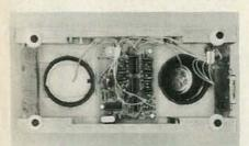
FIG. 7-PC BOARD is mounted, componentside-down, on short standoffs. Switches, hidden by board, are mounted on enclosure.
