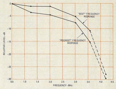
FIG. 1—VIDEO FREQUENCY-RESPONSE of the best and worst videotapes tested differed by almost 5 dB at same frequencies.
