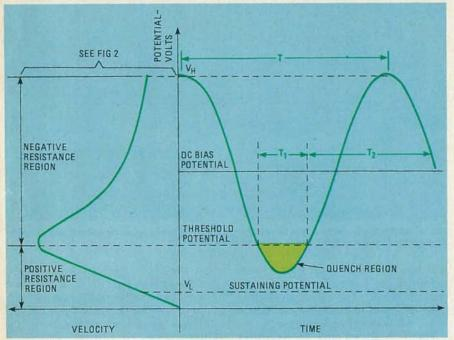
FIG. 7—THE DC BIAS VOLTAGE must be carefully selected so that the total bias drops below V<sub>TH</sub> but remains above the sustaining potential on negative peaks of the RF cycle.
