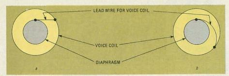
FIG. 7—LENGTHENING the effective span of the voice-coil leads (b) reduces the stress on those leads in the MDR-series headphones.
