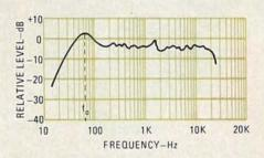
FIG. 5—TYPICAL RESPONSE CURVE for a speaker system. The frequency f<sub>0</sub> is the minimum resonant frequency.
