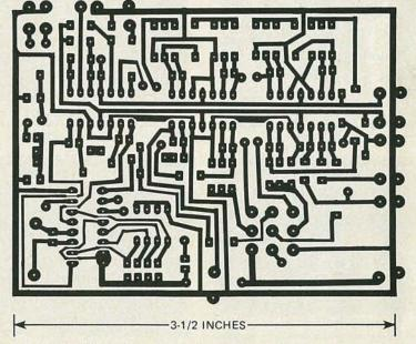
FIG. 5—THIS FOIL PATTERN can be easily reproduced, although the between-the-pin traces near IC4 may require special attention.
