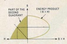
FIG. 3—THE ENERGY PRODUCT is the product of flux density and magnetizing force, and is very different for different materials.
