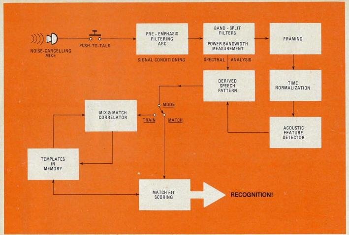
FIG. 1—GENERALIZED block diagram of a speech-recognition system shows how a spoken word is processed so that it can be recognized by a computer.
