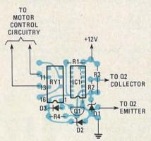
FIG. 94—DETECTOR BOARD is connected to FPT-100 sensor by 18-inch leads. See text for motor-control connections.
