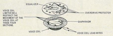
FIG. 9—THE DIAPHRAGM is covered by a small plate that acts as an acoustic equalizer as well as a protective device.
