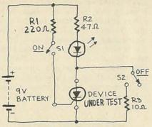
ALL RESISTORS, 1/2 WATT SI & S2: N.O. SPST USE ALLIGATOR CLIPS FOR CONNECTIONS
