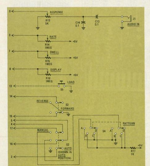
FIG. 3—MAIN FRONT-PANEL switches and potentiometers. Swich S2 is of the "center-off" type.
