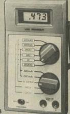
Easy-to-read 0.4"-tall liquid crystal display with convenient low-battery and over-range indicators. Measures up to 500VAC in 4 ranges; 1000VDC in 4 ranges; 200 mA AC and DC current in 3 ranges each; 20 megohms resistance in 6 ranges. Size: 64x34x144" Leads and manual included. Requires 9V battery or AC adapter. 22-198. 79.95 AC Adapter. U.L. listed, 273-1431 ..........4.95
