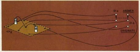
FIG. 10—A DPDT SWITCH, S1, is wired as shown for testing the modern. After testing is complete, rewire the switch to match the schematic.
